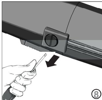
**Note:** The brush must be inserted with its black part directed inside the motor.
