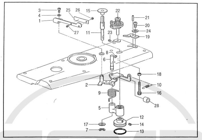
糸ゆるめ関係/Tension release mechanism
