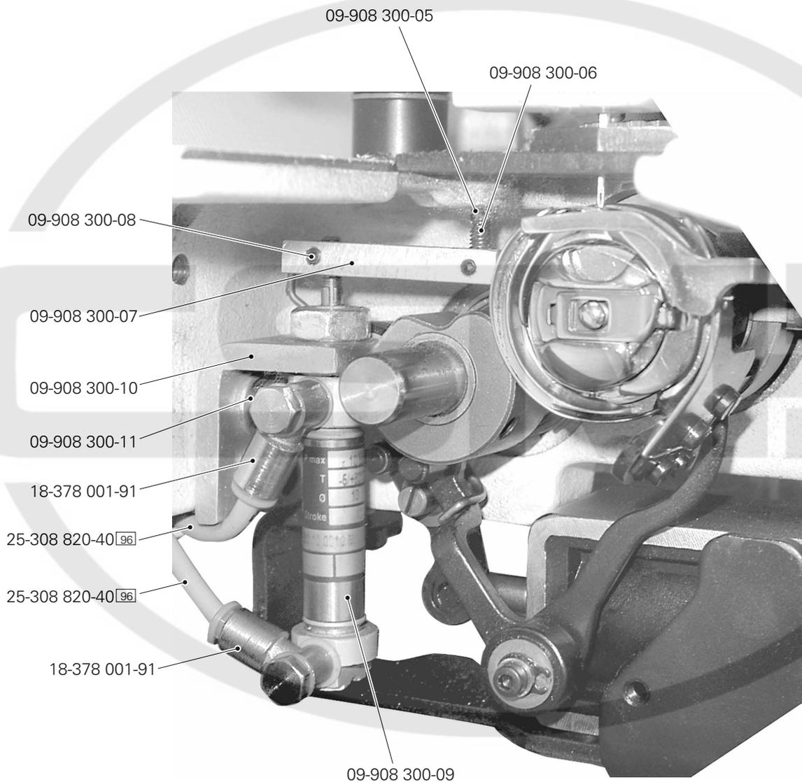
I used M6 X 20 mm counter sunk screws to mount the angle bracket making it much easier to remove. The holes in the casting for mounting the angle bracket must be counter sunk as well. The cylinder is a Bimba 10mm dia and 10 mm stroke. For a part number use the same number as above. The cylinder coming from Germany is a magnet type cylinder. The Bimba is not.
