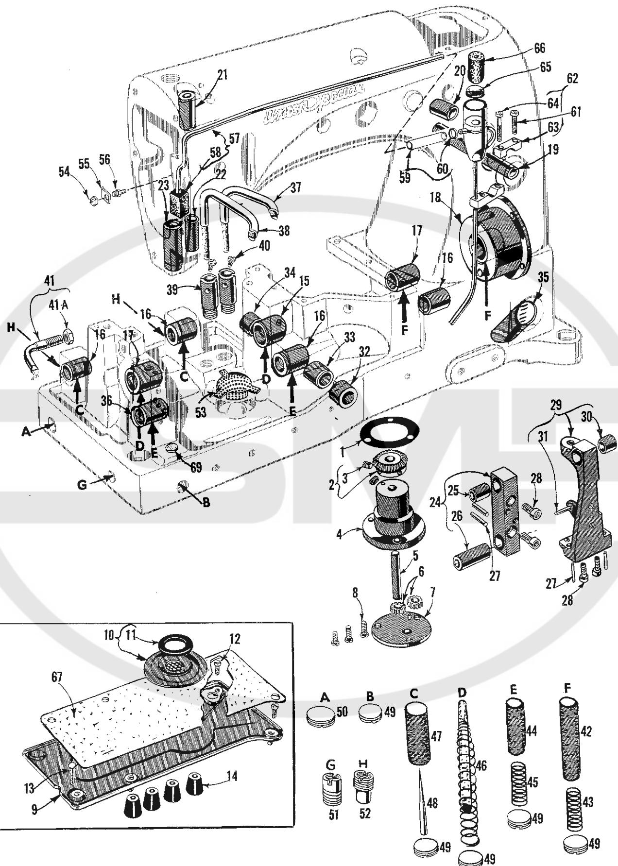
MAIN FRAME, BUSHINGS AND MISCELLANEOUS OILING PARTS
