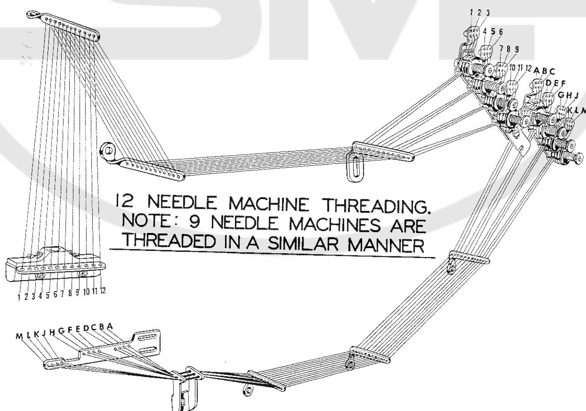
THREADING AND OILING DIAGRAM FOR STYLES 54200 N AND 54200 P
