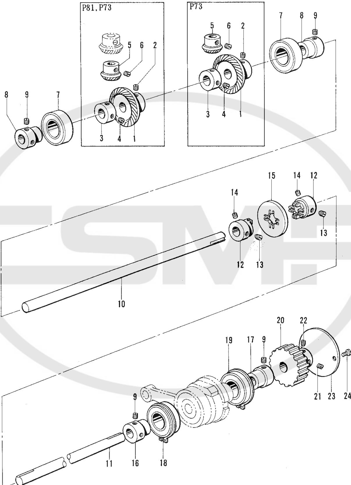
H. 下軸関係/Lower shaft mechanism/Untere Welle/
