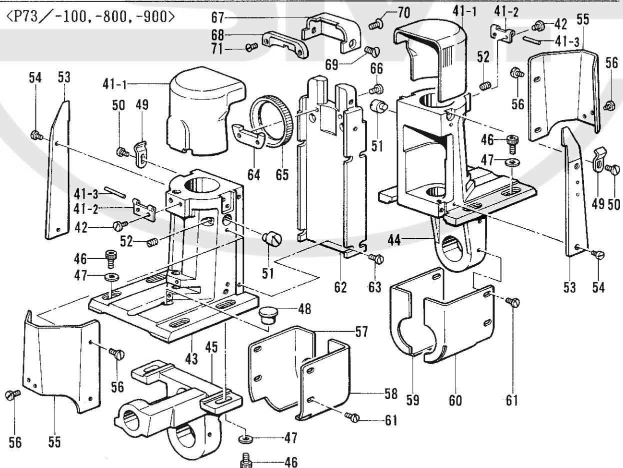
J5. カマ関係/Rotary hook mechanism/Greifervorrichtung/
