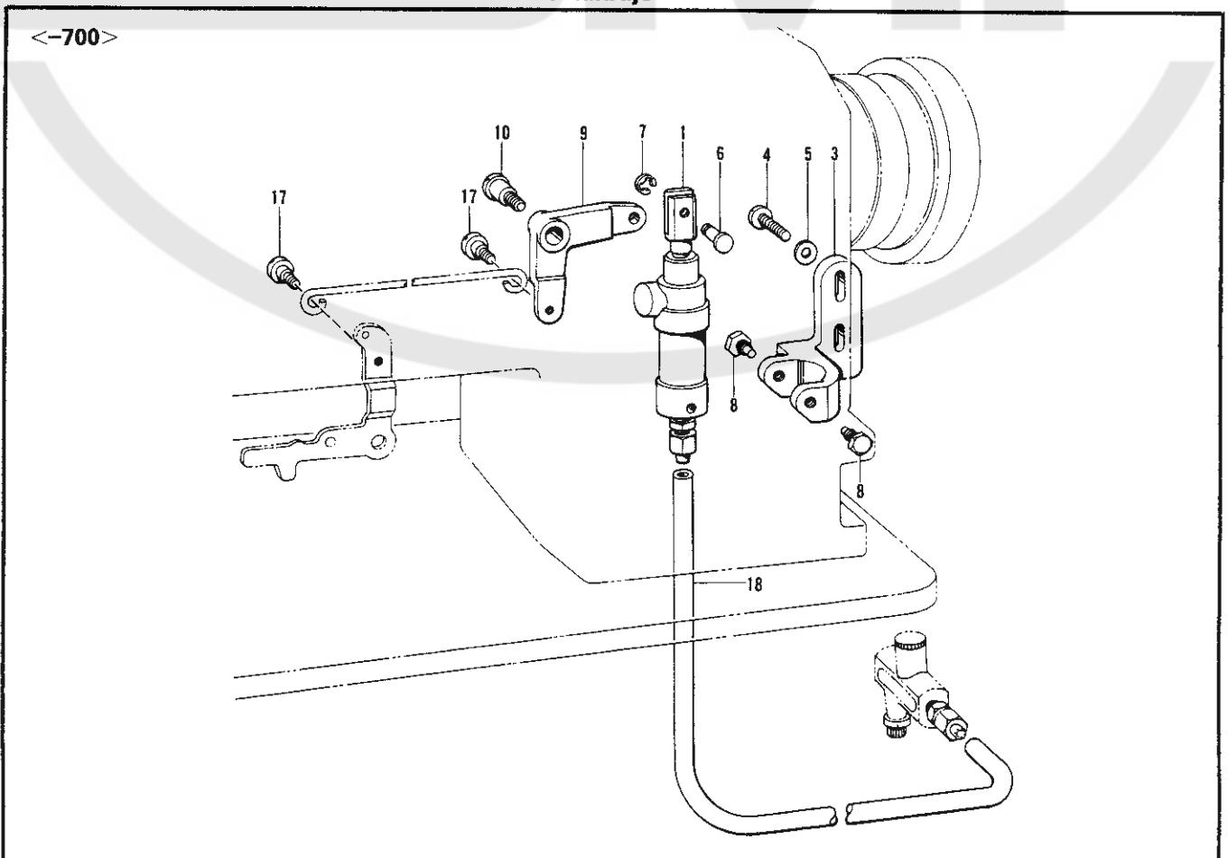
F. 送り軸関係/Feed shaft mechanism/Transport welle/
