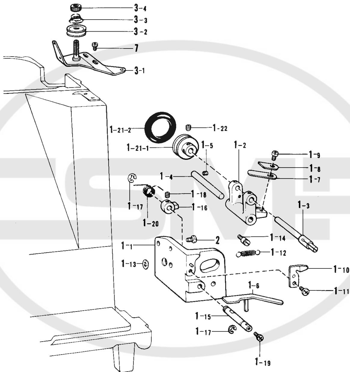
M. 糸巻キ関係 / Bobbin winder mechanism / Spuler
