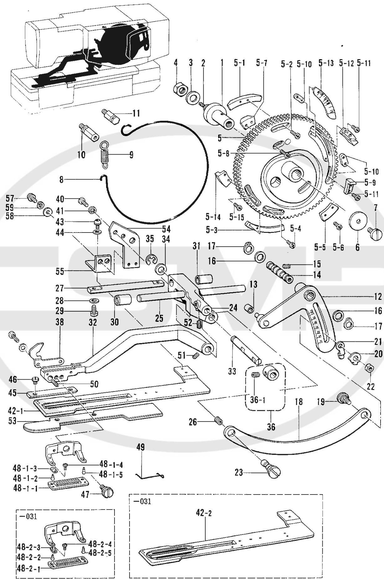
M. 送り関係/Feed mechanism/Transportvorrichtung/
