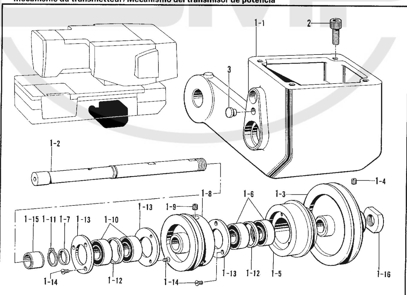
D. 針棒関係/Needle bar mechanism/Nadelstangenvorrichtung/
