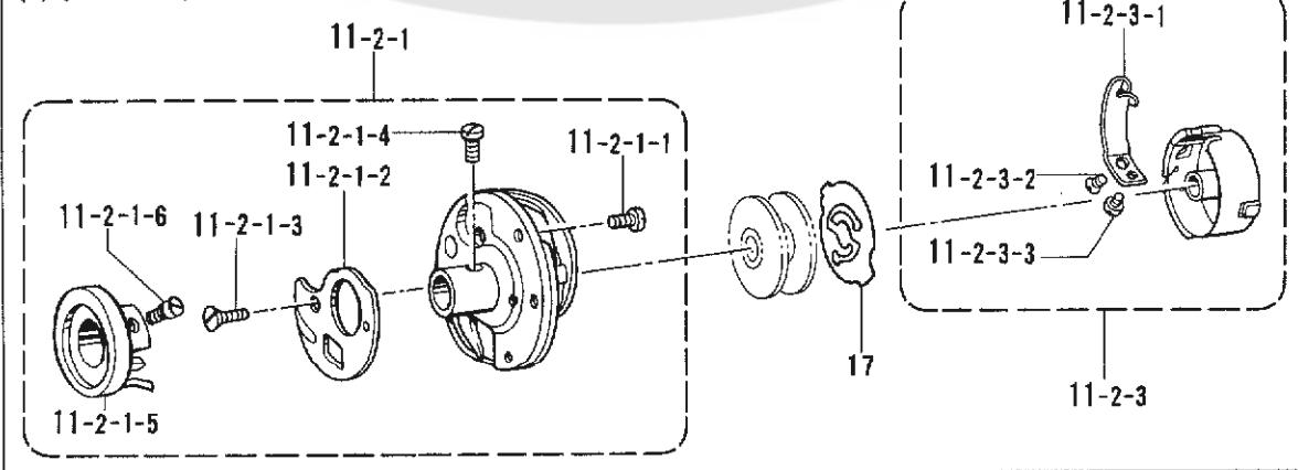
R. カマ関係/Rotary hook mechanism/Greifervorrichtung/
