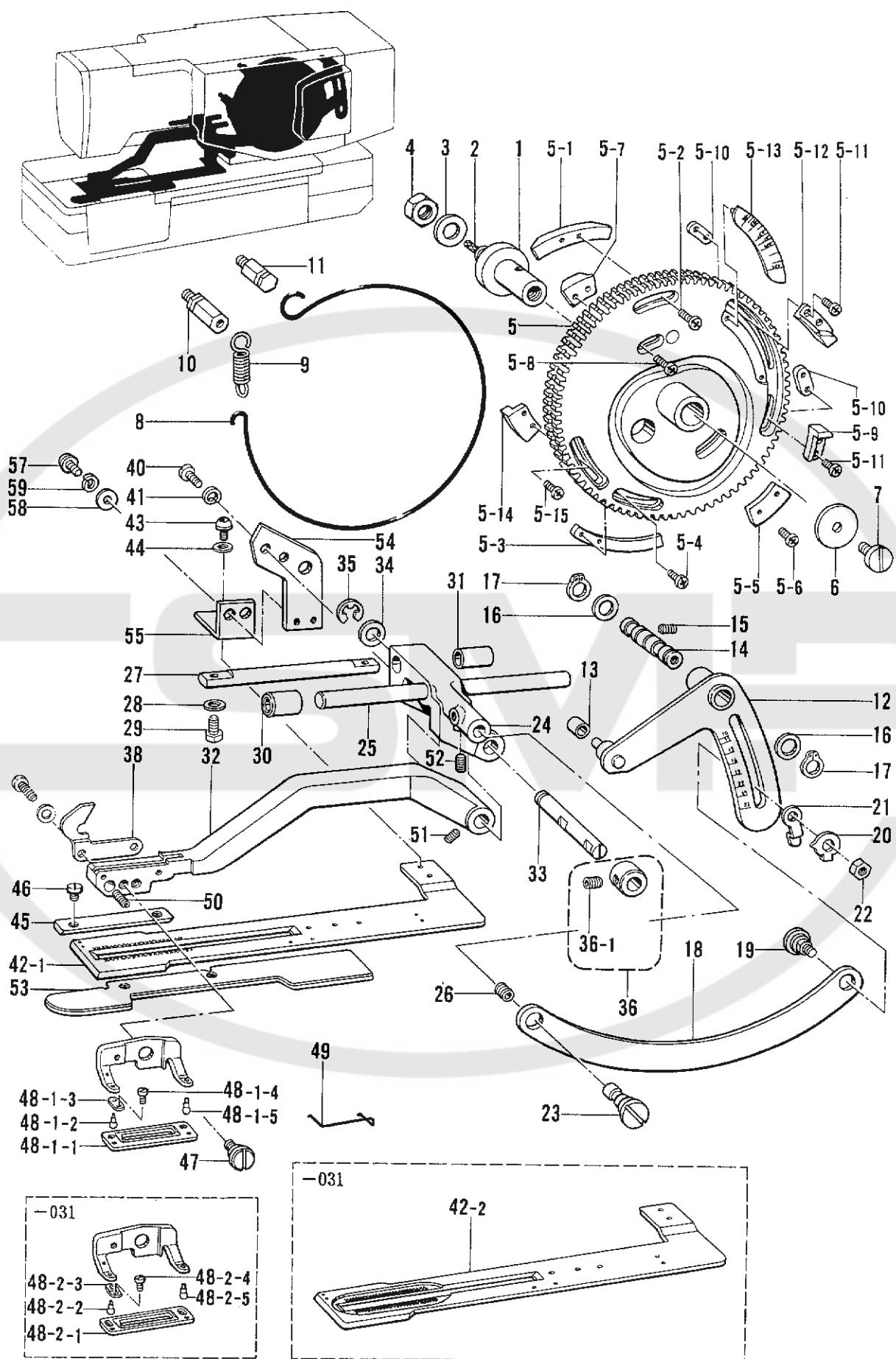
M. 送り関係/Feed mechanism/Transportvorrichtung/
