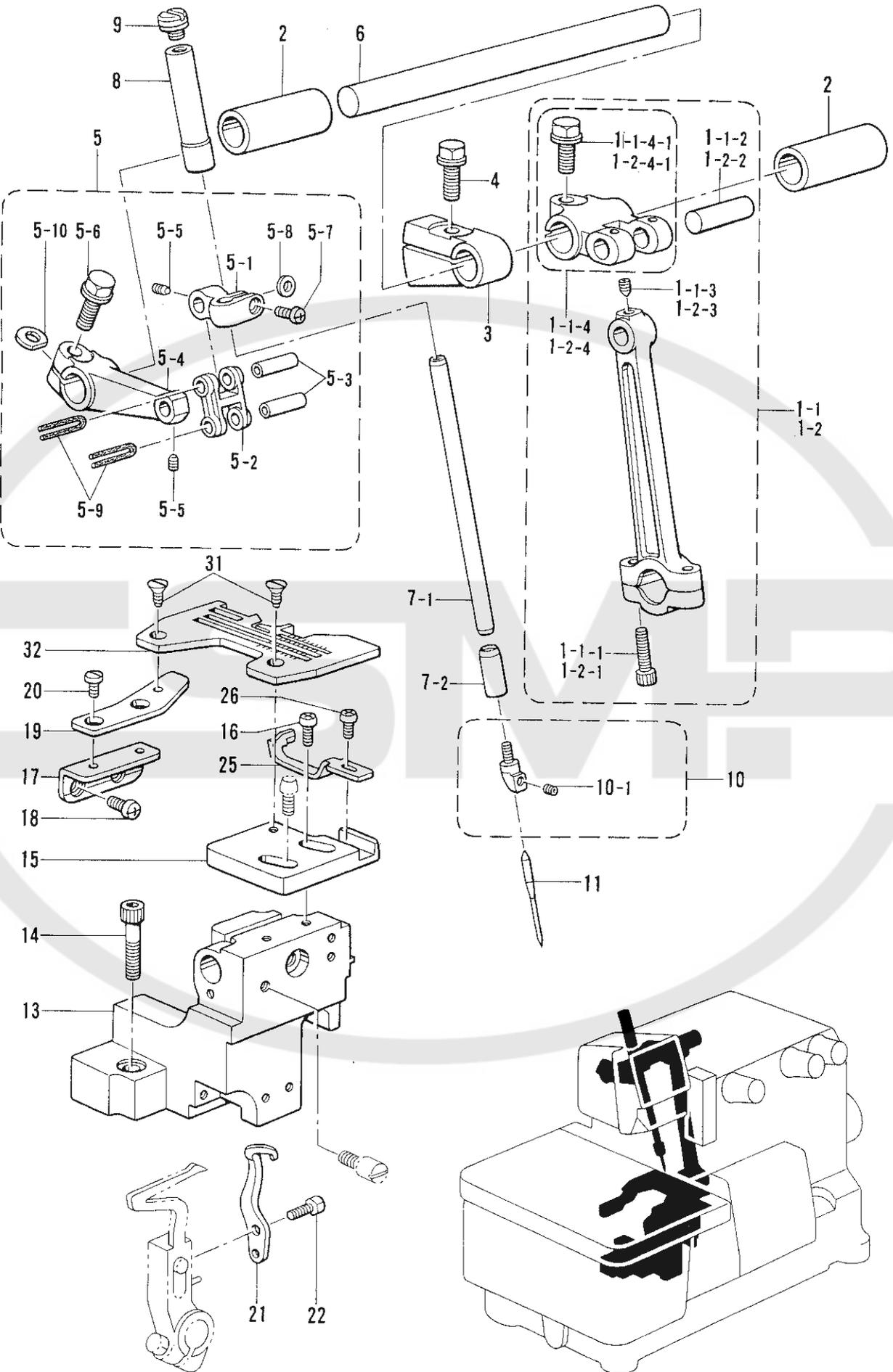
C. 針棒関係/Needle bar mechanism/Nadelstangenvorrichtung/
