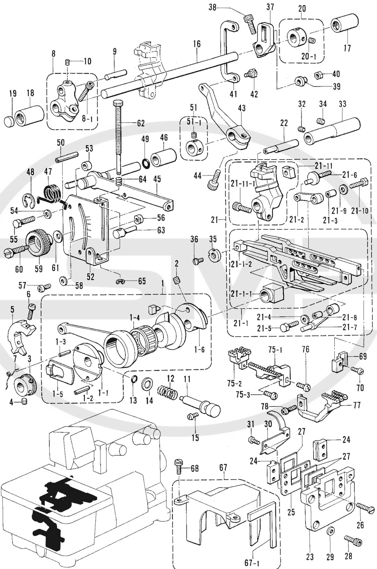
E. 送り関係/Feed Mechanism/Transportvorrichtung/
