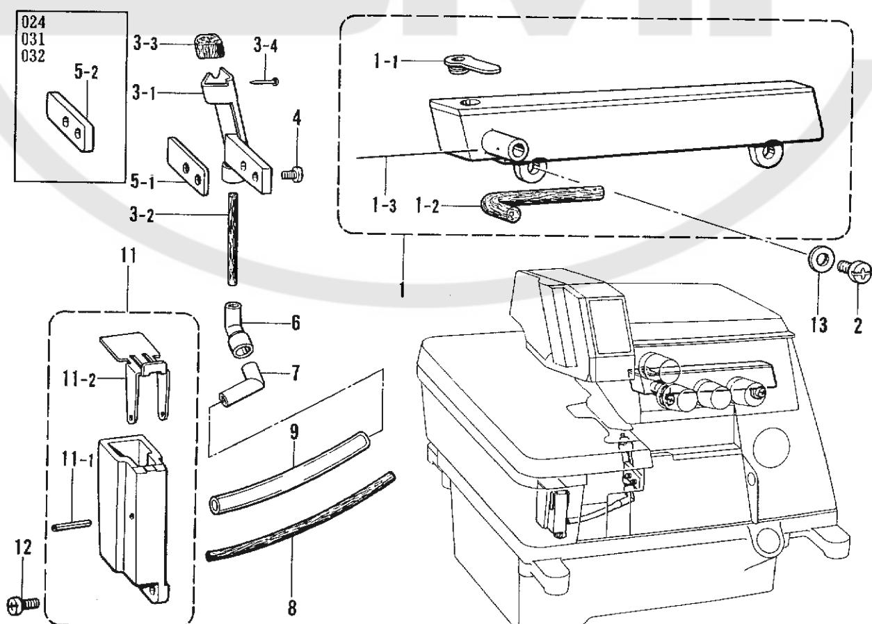
B. 駆動軸関係 / Crank shaft mechanism / Kurbelwelle /
