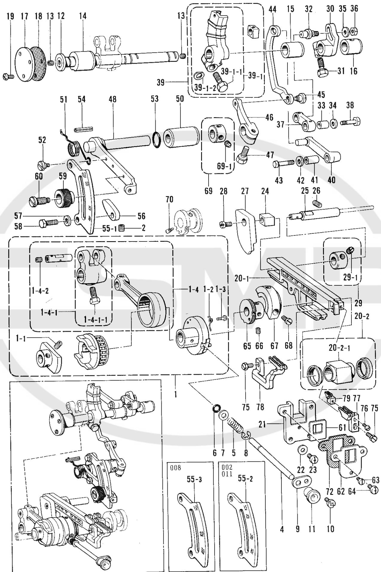
F. 送り関係/Feed mechanism/Transportvorrichtung/
