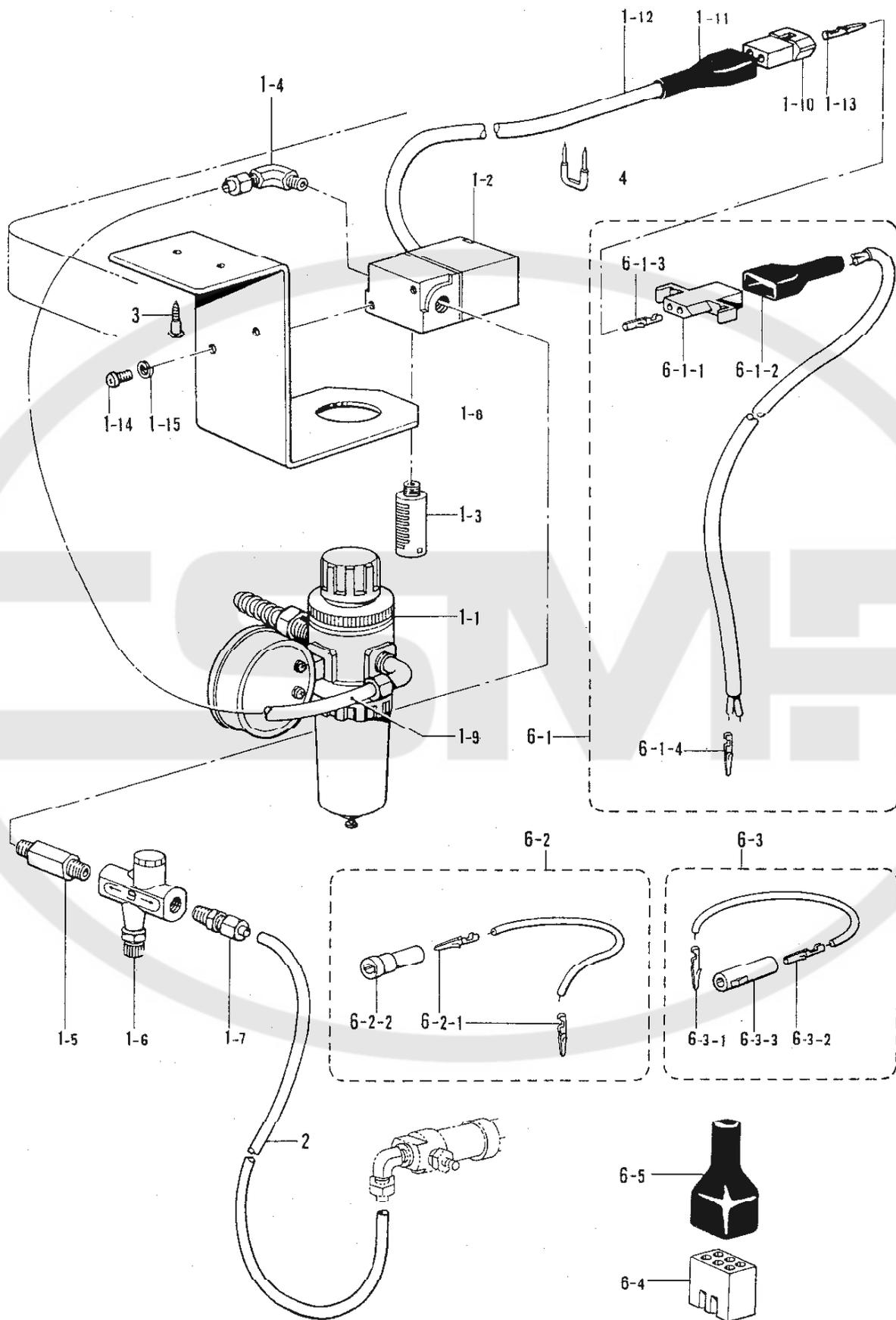
T. 空圧関係/Air pressure mechanism/Luftdruck/
