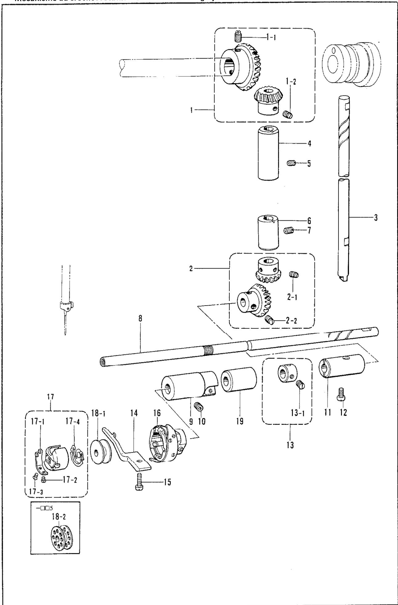
G. カマ関係/Rotary hook mechanism/Greifervorrichtung/
