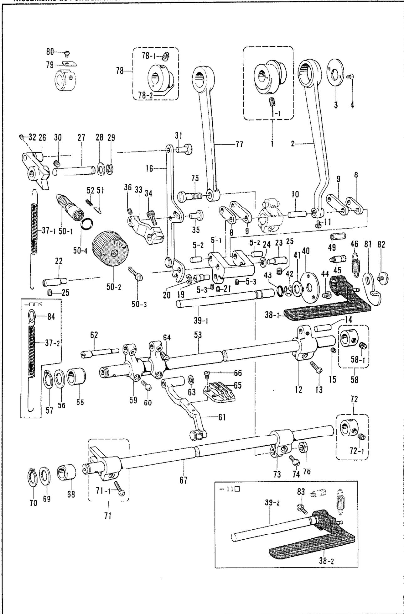
E. 送り関係/Feed mechanism/Transportvorrichtung/
