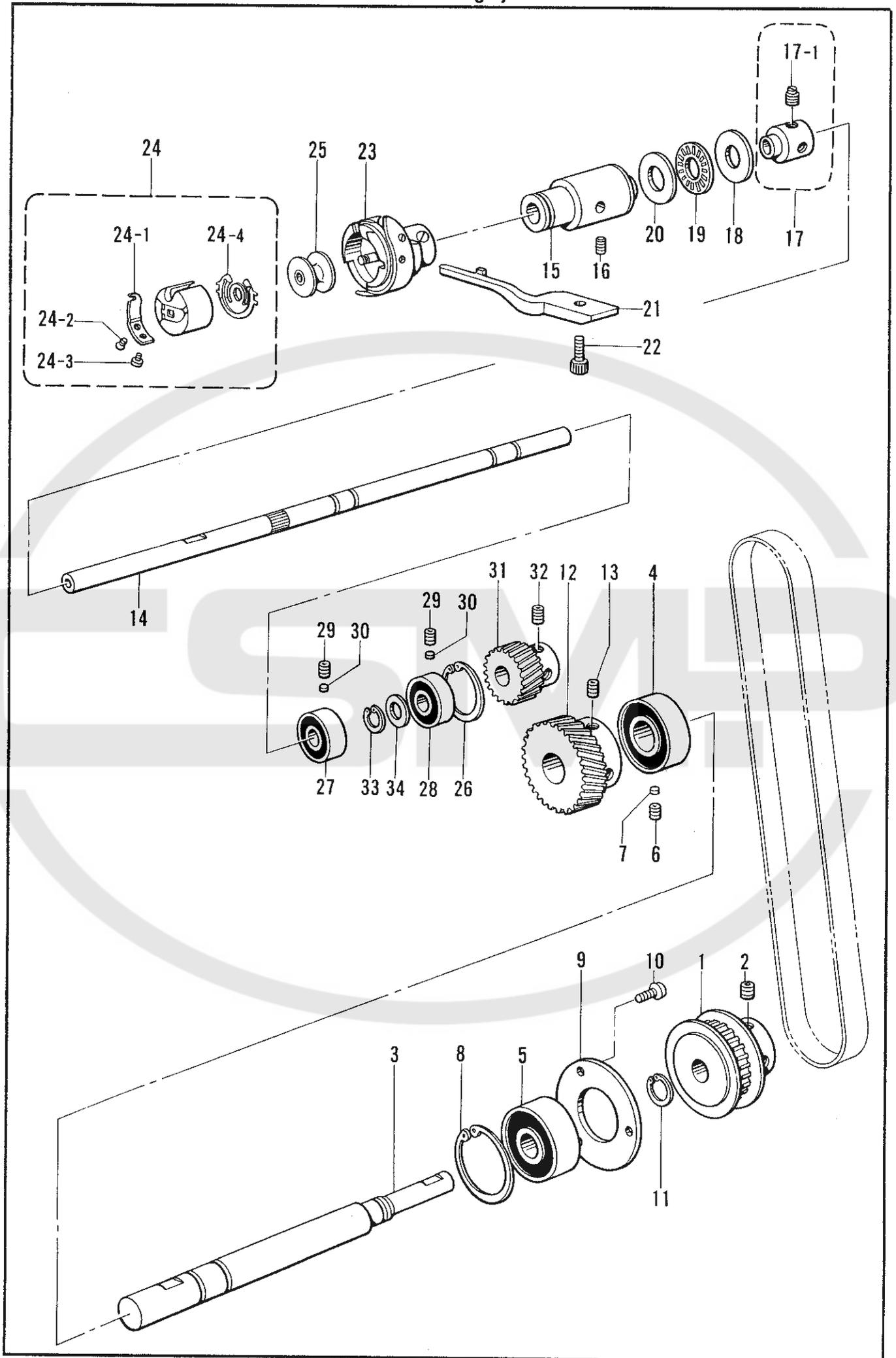
F. カマ関係/Rotary hook mechanism/Greifervorrichtung/
