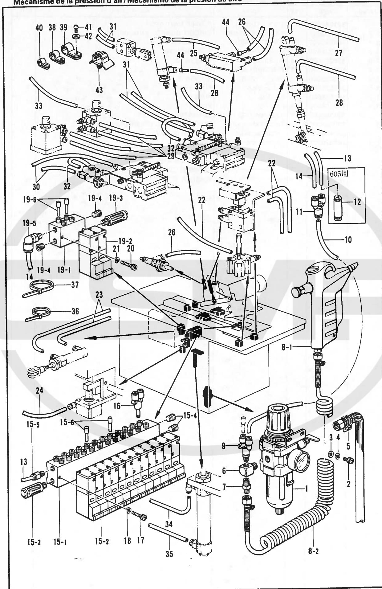
P. 空圧関係/Air pressure mechanism/Luftdruck/
