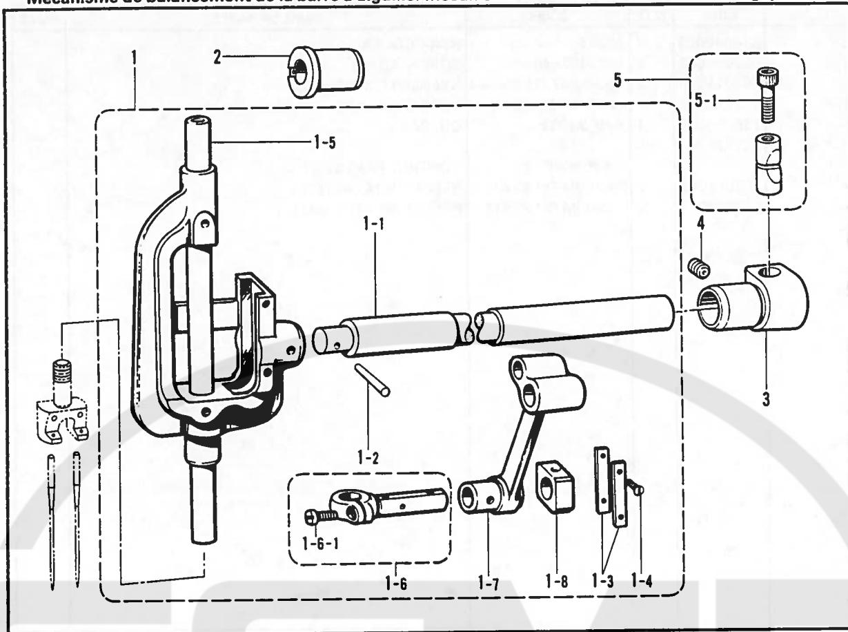
D. 下軸関係 / Lower shaft mechanism / Untere welle /
