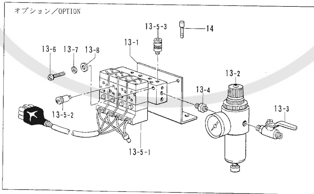
U. 空圧関係/Air pressure mechanism/Luftdruck/
