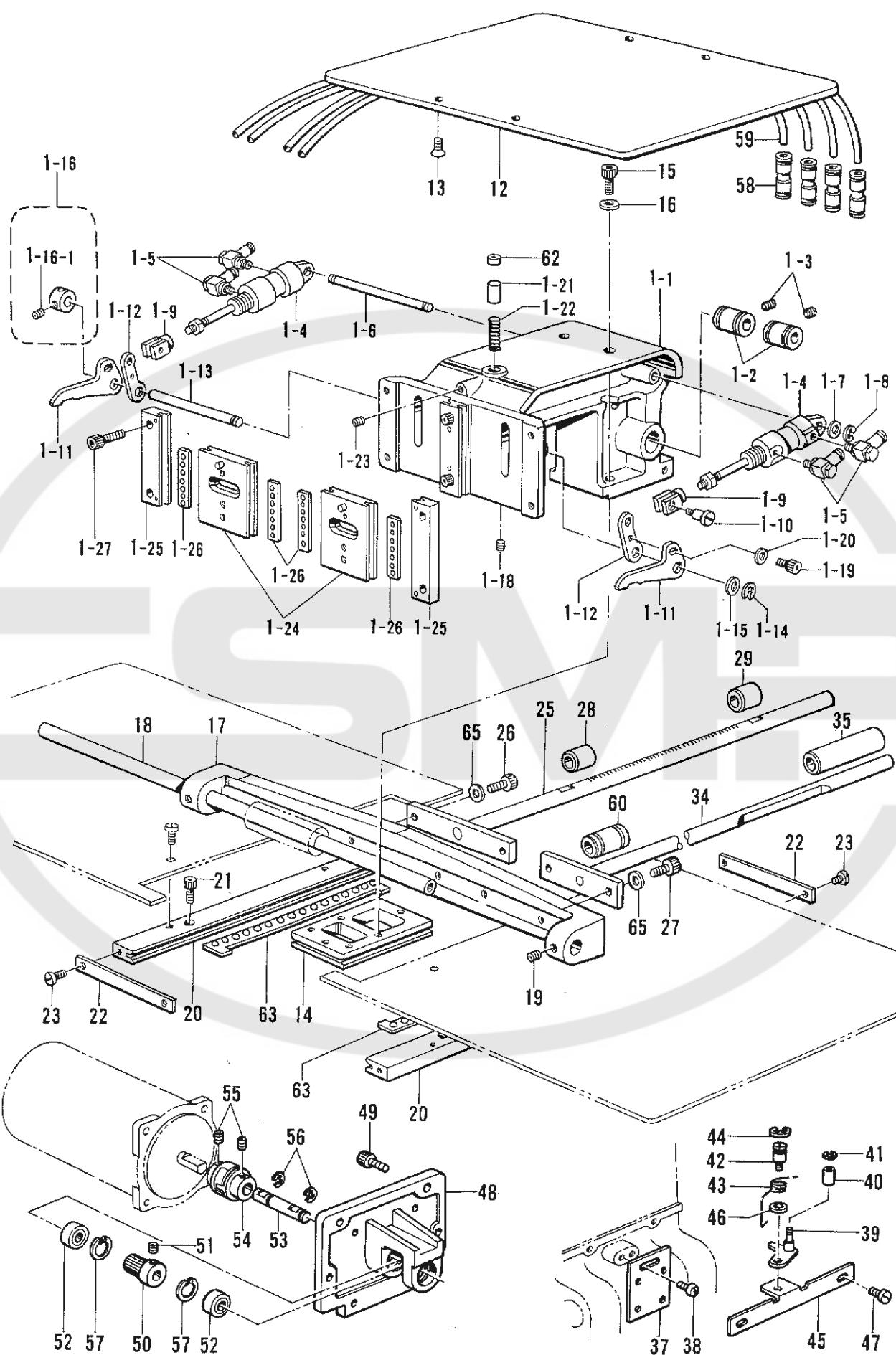
D1. 送り関係/Feed mechanism (1)/Transportvorrichtung (1)/
