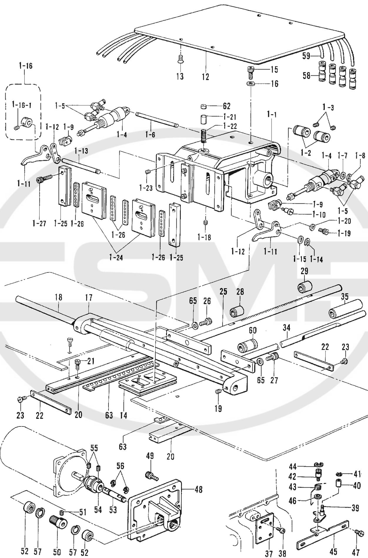
D1. 送り関係/Feed mechanism (1)/Transportvorrichtung (1)/
