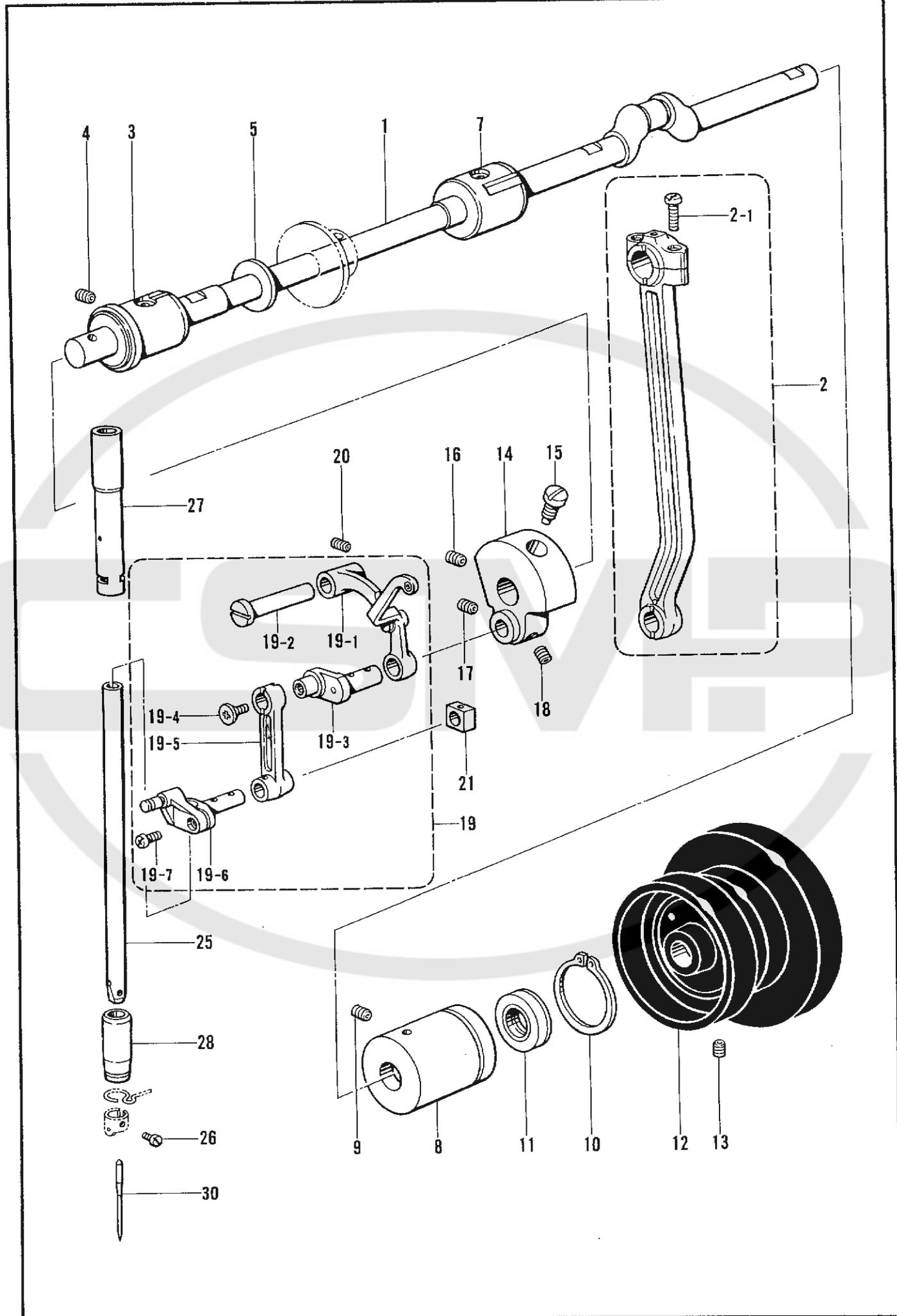
C. 送り関係(1)/Feed mechanism (1)/Transportvorrichtung (1)/
