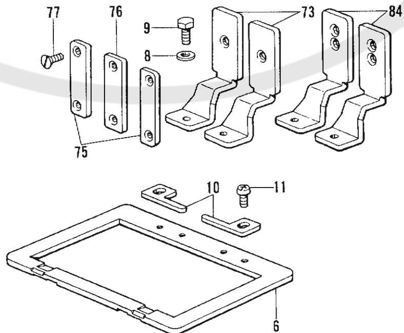
C. 送り関係(1)/Feed mechanism (1)/Transportvorrichtung (1)/
