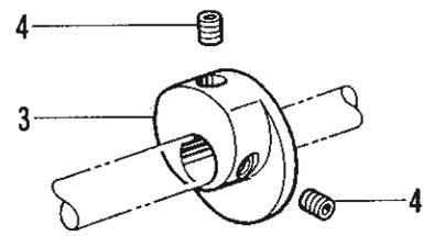
J. 糸巻関係/Bobbin winder mechanism/Spuler/
