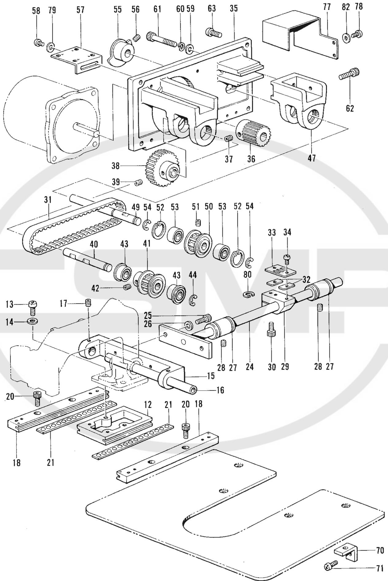
C. 送り関係/Feed mechanism/Transportvorrichtung/
